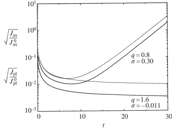
FIGURE 1. Temporal evolution of  $(J_{\text{pl}}/J_{\text{pl}}^0)^{1/2}$  (solid line) and  $(J_{\text{ax}}/J_{\text{ax}}^0)^{1/2}$  (dotted line) for  $\gamma = 0$  at swirl numbers  $q = 0.8$  and  $q = 1.6$ , with  $Re = 667$ .
